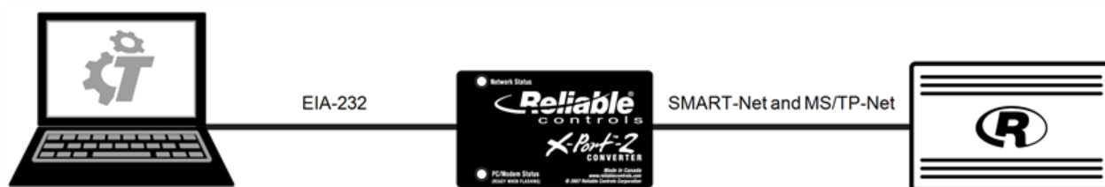
Figure 24: Computer connection to the controller's SMART-Net and MS/TP ports using the X-Port-2
